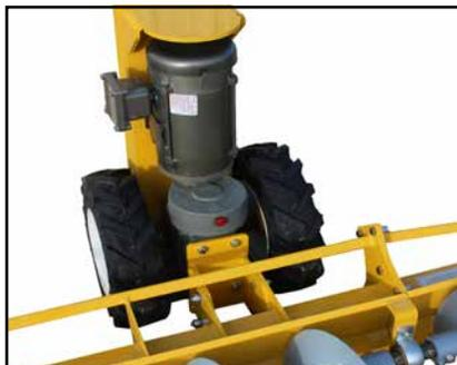
**Weighted Tractor Drive** offers greater traction and has more power to help drive the sweep into the grain. Weight on the drive is adjustable.
