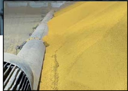
**Forward Motion Auto Drive for True Zero Entry** is standard to manage grain avalanches and compacted grain without the need to reverse.
